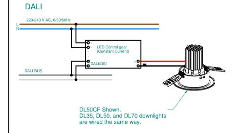
Note: Ensure that the ballast output current and voltage range match the requirements of the downlight specified.
