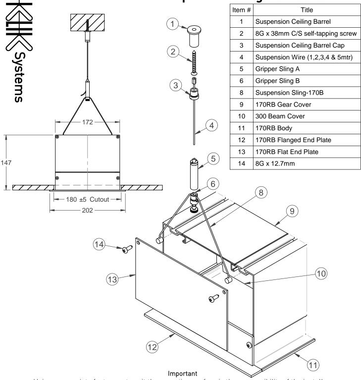
Using appropriate fasteners to suit the mounting surface is the responsibility of the installer.
