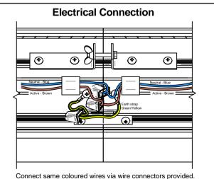
Ensure wires are pushed in tight and check they are secure.
