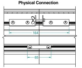
After pins are slid into place, fasten the wing nut and screw as shown. Fasten the flat bar across the join as shown. Make sure positive pressure is applied, to tightly bring together the joining units.
