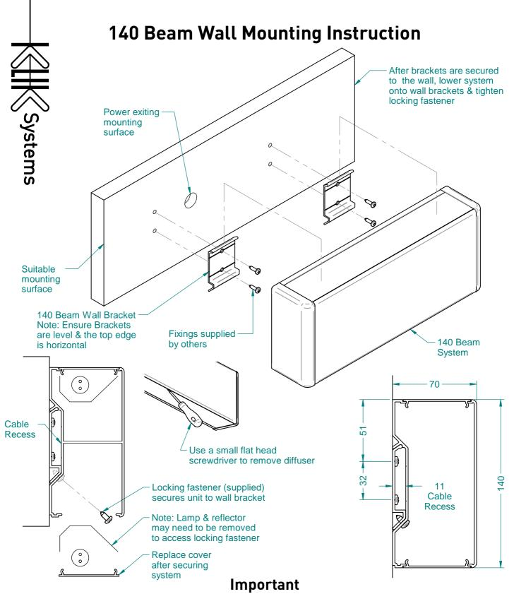
Using appropriate fasteners to suit the mounting surface is the responsibility of the installer. Units should be supended at two points at all times to avoid the over-loading of fasteners.
