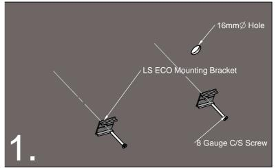
Determine position of fitting, Drill 16mmØ hole for wiring 2mm inside of end of lamp unit final position.
