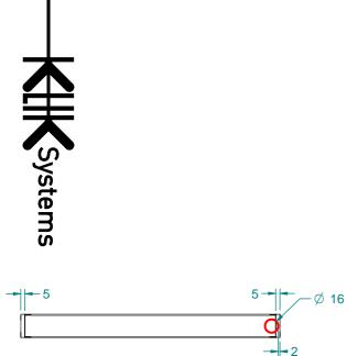
Illuminated area is 10mm less than overall length of Lamp Unit
