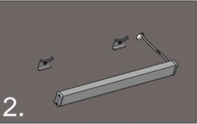
Connect 24V wiring and push lamp unit into place.
