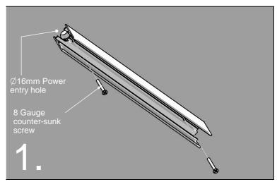
Determine position of fitting and drill appropriate fixing holes and Ø16mm power entry hole.
