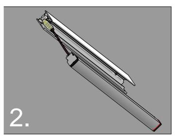
Connect 24V power leads and snap lamp unit into place. Tap gently until lamp unit is centrally located in body.
