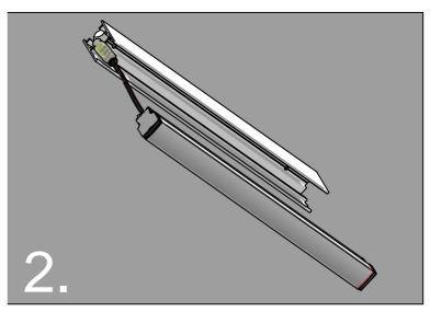
Connect 24V power leads and snap lamp unit into place. Tap gently until lamp unit is centrally located in body.
