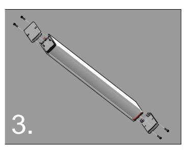
Using a 1.5mm Allen Key, screw on endcaps to finish.
