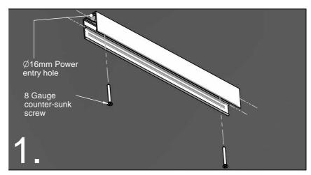
Determine position of fitting and drill appropriate fixing holes and Ø16mm power entry hole.
