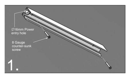
Determine position of fitting and drill appropriate fixing holes and Ø16mm power entry hole.
