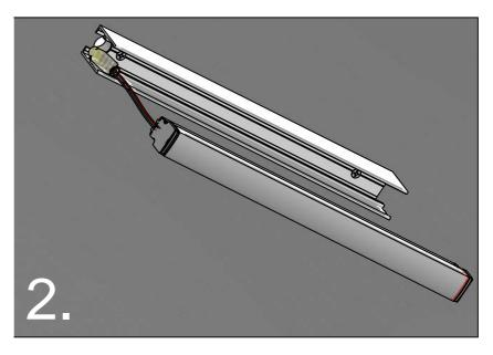
Connect 24V power leads and snap lamp unit into place. Tap gently until lamp unit is centrally located in body.
