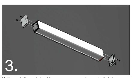
Using a 1.5mm Allen Key, screw on endcaps to finish.
